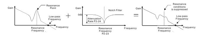
Use Low-pass Filter to suppress resonance
