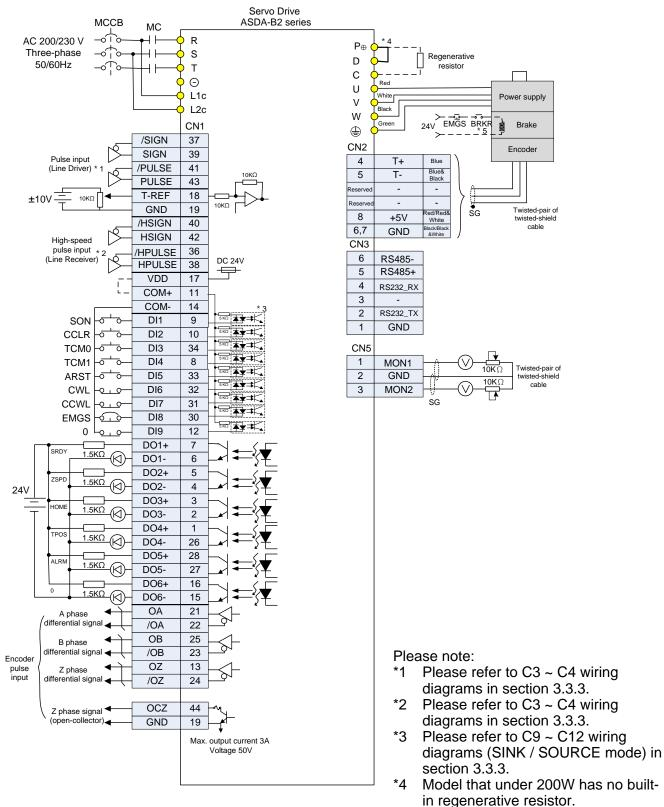
\*5 The brake coil has no polarity.
