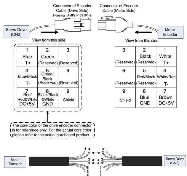
If the users do not use the connector (without housing) and connect the cores from the cable for wiring, please follow the terminal identification and core number of encoder connector shown in the above table to complete the wiring. The users need to connect core #1 to core #1, core #2 to core #2 and so on. To ease connection and to avoid wiring error, it is recommended to number the cores first in accordance with the terminal identification and then conducting the wiring.
