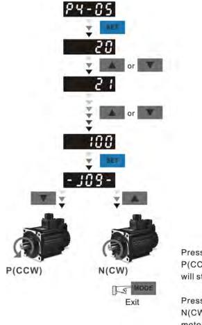
Pressing key and the servo motor will run in P(CCW) direction. After releasing UP key, the motor will stop running.
