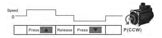
If the servo motor does not rotate, please check if the wiring of U, V, W terminals and encoder is correct or not.
