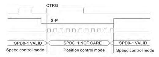
Figure 1. : Speed / Position Control Mode Selection
